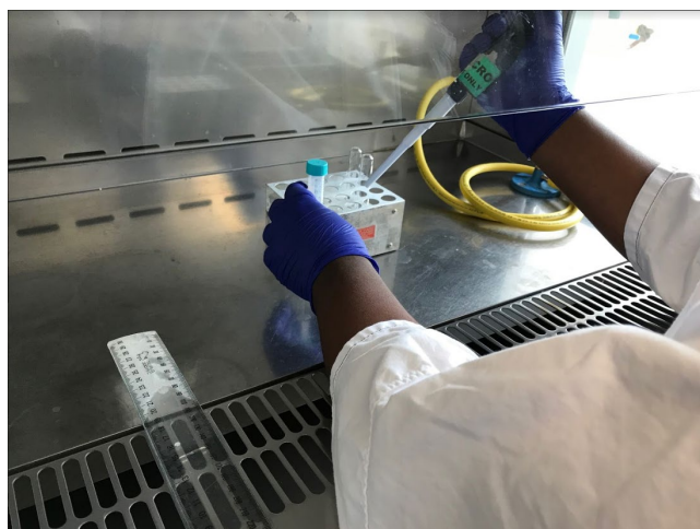
Figure 2: Demonstration of working within the work zone of the cabinet, showing a 10 cm distance from the front grille (ruler provided to show 10 cm distance).
